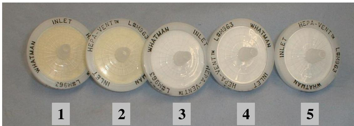
Figure 1 The five  $\mu\text{m}$ -filters for tests 1 to 5 performed July 20, 2001. For black-white prints: the filters 1 and 2 have a clear yellow colour whereas filters 3, 4 and 5 are white.
