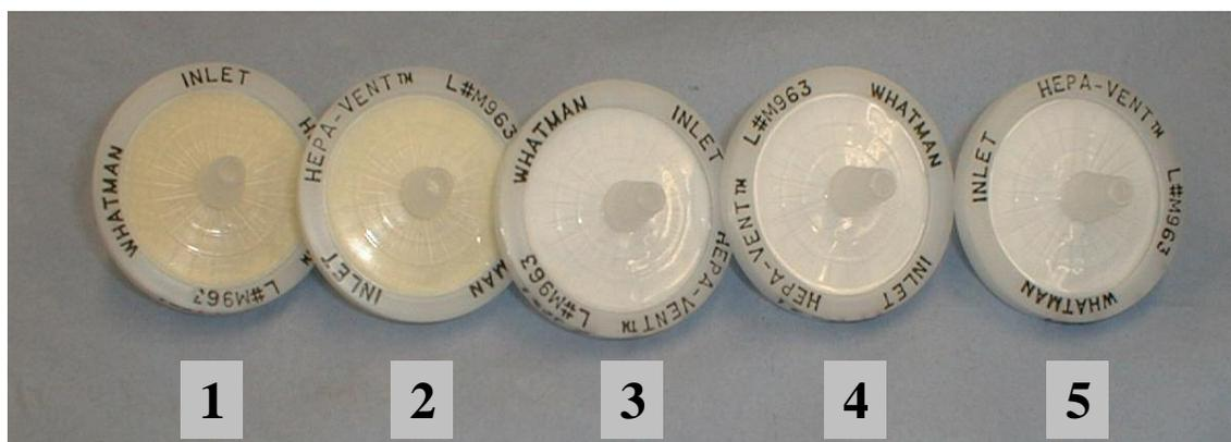
Figure 1 The five  $\mu\text{m}$ -filters for tests 1 to 5 performed July 20, 2001. For black-white prints: the filters 1 and 2 have a clear yellow colour whereas filters 3, 4 and 5 are white.
